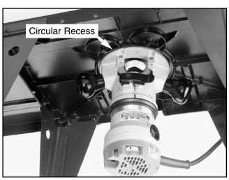
Figure 7. Router positioned correctly for "Method 1" installation.
